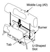
Figure 25 - Installing Middle Log (#2) (CCL3930PR/NR Shown)
